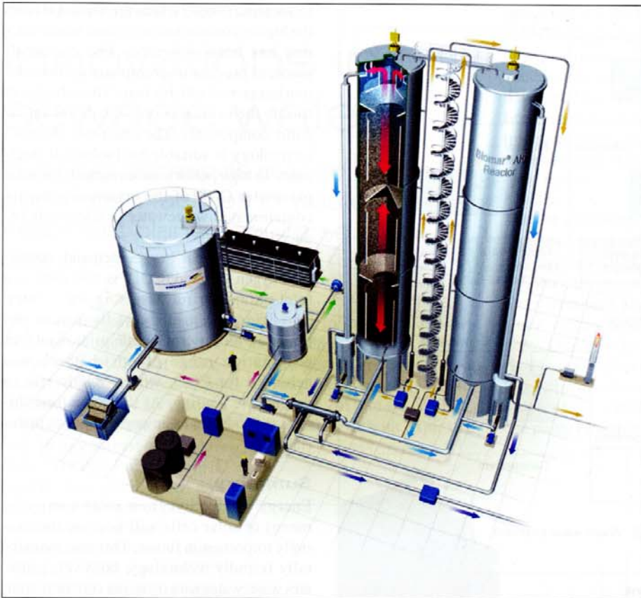
Diagrammatic view of the anaerobic Biomar® process
